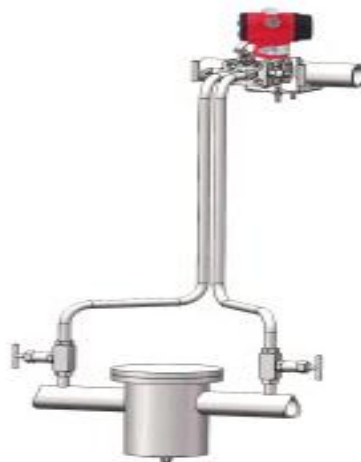
Pipe Differential Pressure Measurement
